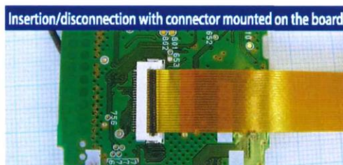
Circuit board inspection (in place of disposable flexible wiring)
