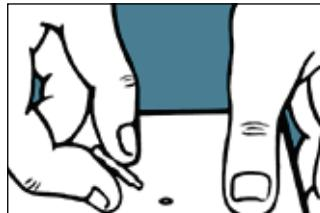
1. Insert receptacle into the drill hole.
