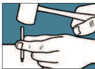
3. Tap the top of the tool with a small plastic hammer until the receptacle is seated at the proper height. The press ring keeps the receptacle in place.
