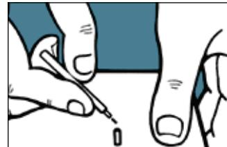
2. Insert tip of RIT tool into the top of the receptacle and, with slight hand pressure, seat the receptacle into the drill hole until resistance is met.
