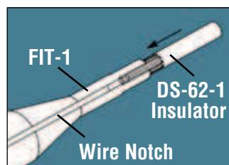
1. Insert insulator, knurled end first into tip of FIT tool.
