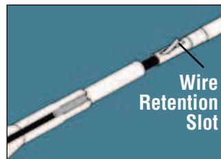
3. Hold wire firmly against tool with forefinger. Insert protruding wire into termination end of W-4 receptacle. Release grasp on wire and push insulator onto end of receptacle, completing termination.
