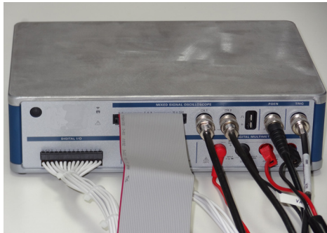
Detail of the Measurement Unit (P/N AD539) included in the 6TL-08 UNIVERSAL, with FGEM, DMM, Scope DIO and Logic Analyzer.
