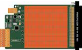
YAV90077 6200.77 21-Channels 1-wire 6A 250 V Two fault insertion buses ➤ Switching up to 250 W. ➤ Carry current up to 6A ➤ CAN bus controlled ➤ Form factor G
