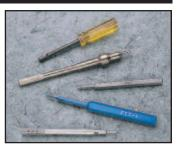
Probe Insertion/Extraction Tool (PIE) Receptacle Insertion Tool (ARIT-25) Receptacle Insertion Tool (RIT) FASTITE® Insertion Tool (FIT) Adjustable Receptacle Insertion Tool (ART)
